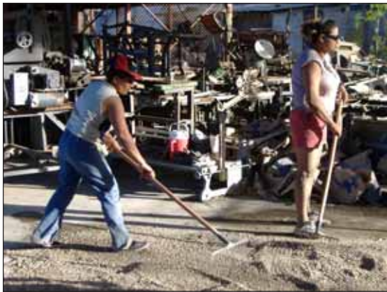
Women working with the material to make light-weight concrete blocks
